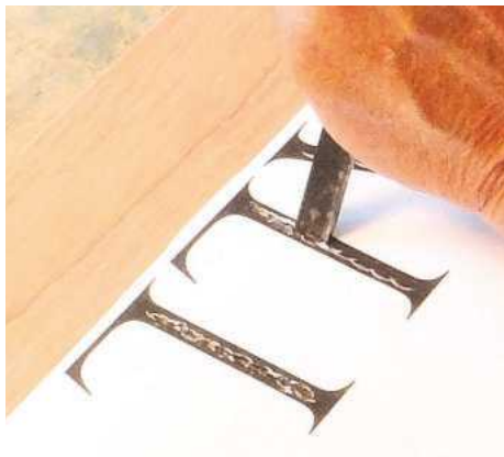
A gouge, not a chisel, is used to begin the straight cuts because the curve of the blade severs the fibres on either side and produces a clean cut. The first touches are a little timid as a central channel is established
